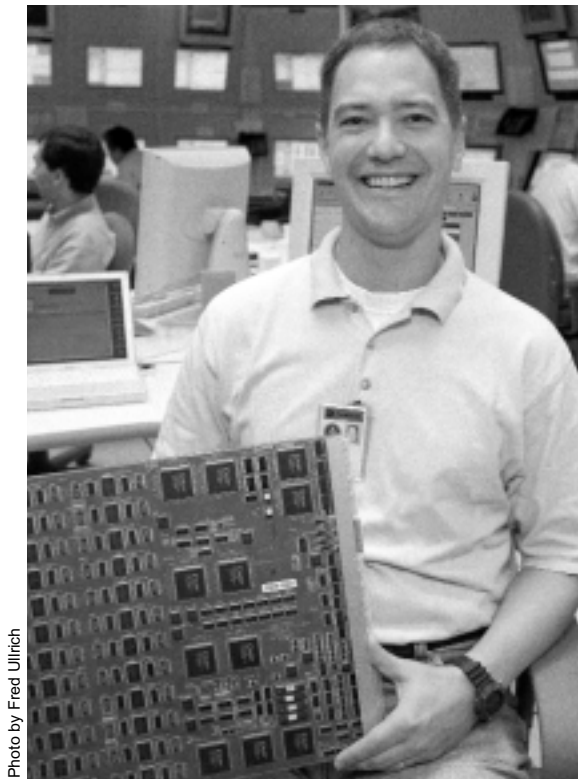
Kevin Pitts and collaborators at the University of Illinois constructed an electronic "extrapolation system" for the trigger system of the CDF detector.
